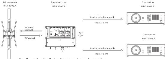
Configuration for 2 simultaneous channel operation:
