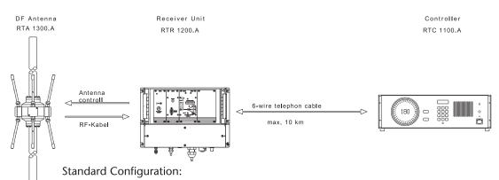
The system operates in "remote mode". The direction finding antenna is installed remotely from the controller, at a location favourable for direction finding. Receiver, demodulator and antenna control module are integrated in the receiver unit located at the antenna position. They are connected to the controller by means of a 6-wire line.
