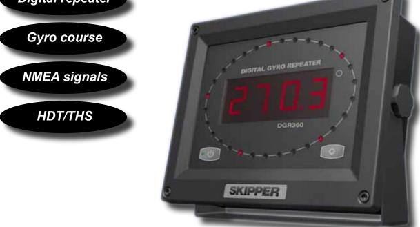
DGR 360 is a digital gyro repeater that displays the Heading Angle in the LED segment display and indicates the Direction of Turn with 30 dual-color surrounding LED's, changing from green to red colour depending on the direction of turn.
